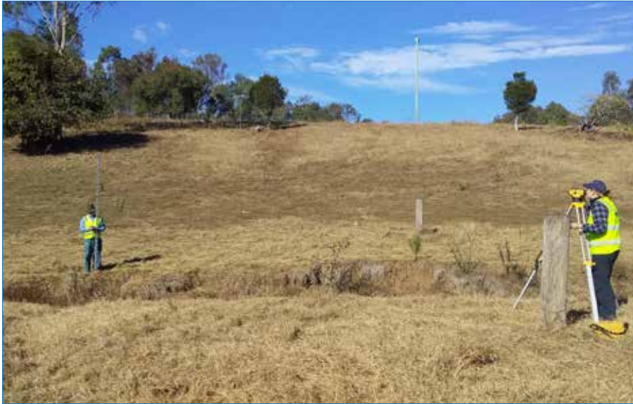
Photo 2 Survey the level crest.
